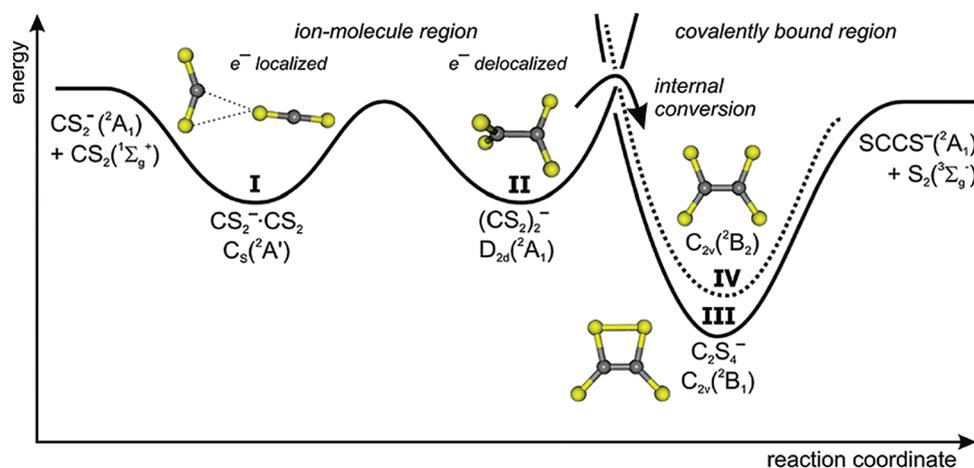
**Figure 4.** Proposed mechanism for isomer conversion of  $(\text{CS}_2)_2^-$  anions (see text). Species I ( ${}^2A'$ ) is mainly produced in the supersonic expansion and accumulated in the ion trap. At 16 K, the internal energy of species I is too small to overcome the isomerization barrier leading to species II ( ${}^2A_1$ ). At 100 K, species I and II are in equilibrium. At 200 K, species II is transformed via internal conversion to species III ( ${}^2B_1$ ) and IV ( ${}^2B_2$ ).
